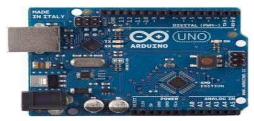
A microcontroller (sometimes abbreviated  $\mu C$ , u C or M C U) is a small computer on a single integrated circuit containing a processor core, memory, and programmable input/output peripherals. Program memory in the form of NOR flash or OTP ROM is also often included on chip, as well as a typically small amount of RAM. Microcontrollers are designed for embedded applications, in contrast to the microprocessors used in personal computers or other general purpose applications.
