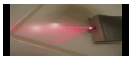
The beam of a laser gun is easily aimed at a target, and scanned across the front grille area at a typical 400 to 600 feet. At those distances, the laser beam is about 12" to 22" wide, depending on manufacturer of the laser gun. Even if you had an excellent radar detector up in the windshield, it probably would not detect the laser beam down on the front grille of target, due to how narrow the beam is. Laser = Light Amplification by Stimulated Emission of Radiation.
